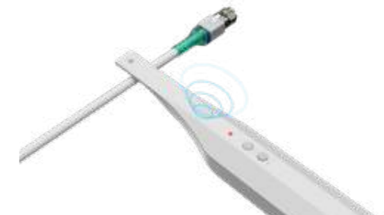
Supported audio cable tracing method
