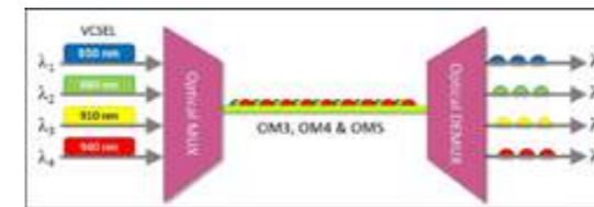
Figure 1: SWDM with Four Wavelengths in MMF
